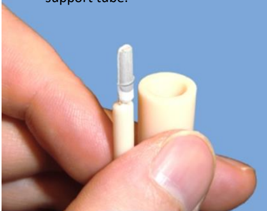
Fig. 1. Tip of the MOSE assembly next to a ProboStat™ sample support tube.
