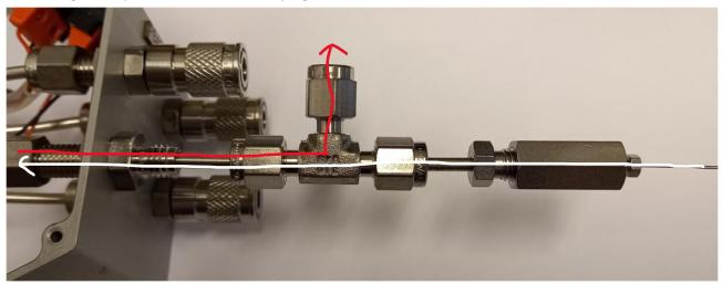
The 1/8" to 1/32" adapter must be bored through to allow the 1/32" line to continuously run all the way through.
