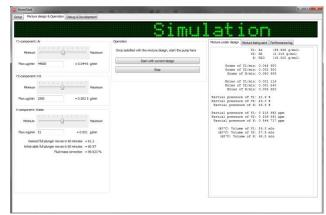
The HumiStat software connects to the humidifier from a Windows PC (not included) with an USB cable (included). The software allows user to select gases from the available pool, and allows the user to design a mixture with specific partial pressures of the components and a segment program.
