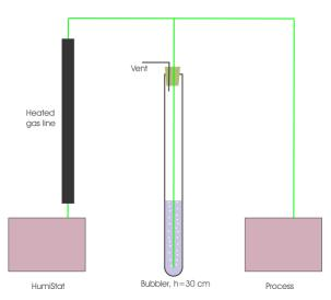
For example 30 cm column with fluid of 1.86 density gives  $0.3m * 9.81 \text{ m/s}^2 * 1860 \text{ kg/m}^3$  = pressure in pascals = 0.055 bar over atmospheric pressure.
