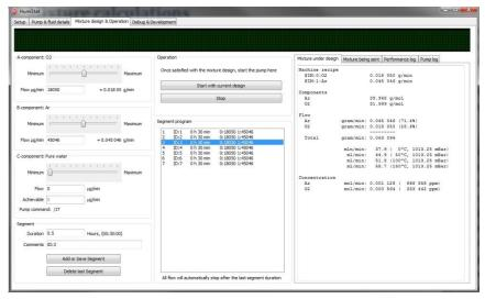
The desired mixture is designed and executed on this view. It is possible to change the amount of any of the three components within the range specific for the instruments, as defined during order.
