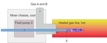
The fluid (component C) is injected to the heated gas through 1/16 inch stainless steel tube. This tiny tube enters the heated gas line tube and the two tubes overlap in the hot zone. When adding large amounts of fluid, the fluid flows into the heated gas line and evaporates there.
