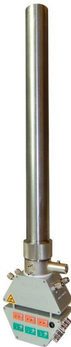
Picture 8. ProboStat™ assembled for high pressure measurements.
