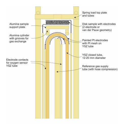
**Figure 1.** Suggested schematical setup of ProboStat with YSZ sensor tube as support tube. Measurements on disk sample can comprise up to 4 wires (e.g. 2-electrode or van der Pauw measurements) provided sensor connections are taken out through usused TCT thermocouple feedthrough. Outer enclosing tube, outer gas supply tube, thermocouple, and base unit are not shown for clarity.
